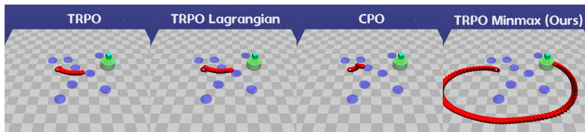
Figure 1: Example trajectories of prior work—TRPO (Schulman et al., 2015) (left-most), TRPO-Lagrangian (Ray et al., 2019) (middle-left), CPO (Achiam et al., 2017) (middle-right)—compared to ours (right-most) in the Safety Gym domain (Ray et al., 2019). For each, a point mass agent learns to reach a goal location (green cylinder) while avoiding unsafe regions (blue circles). The cyan block is a randomly placed movable obstacle. Our approach learns safer policies than the baselines, and works by simply changing the rewards received for entering unsafe regions to a learned penalty (keeping the rewards received for all other transitions unchanged).
